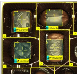
Part location and assembly verification
